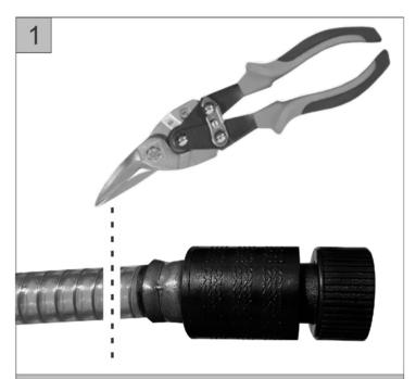
Cut off the old connector. Do not leave reinforcing wire exposed.
