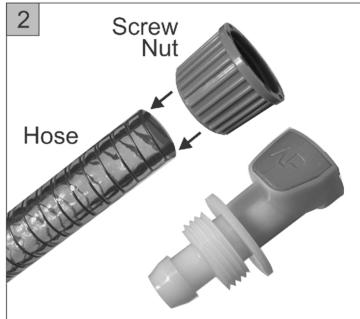
First slide threaded tightener Screw Nut on to Hose.
