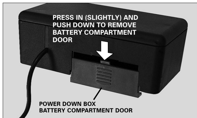
FIGURE 2: Power down box battery compartment door removal.
