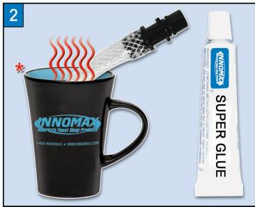
Heat a cup of water to dip the end of the hose in to help stretch the hose around the existing pump port. Quickly dry the hose off to apply the super glue.
