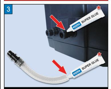
Apply the super glue adhesive to the inside open end of the hose adaptor & also to the outside of the pump port. Next slide the open end of the hose over the port on the pump.
