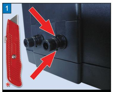
The first step in the process is to cut the top and bottom lock nipple making sure the port is as smooth as possible. Next remove the rubber ring washer from the pump port.
