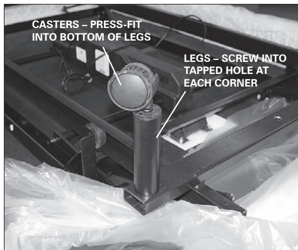
FIGURE 1: Leg and caster installation.
