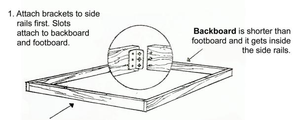
**Footboard** is longer than backboard and it goes in front of side rails.
